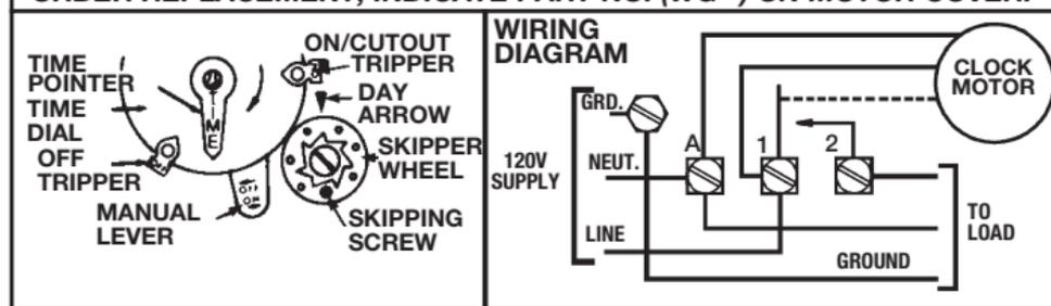
**WIRING INSTRUCTIONS:** Remove 1/2 inch of insulation from wire ends. Tighten terminal screws firmly (2-18 in-lbs). Use solid or stranded COPPER conductors only. May use two wires of the same size and type.
